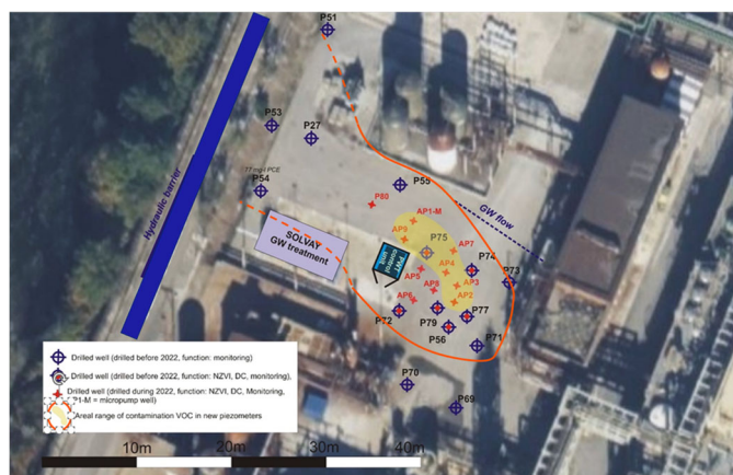
Figure 8. Pilot site of ENB showing contamination, ENB treatment area as well as treatment and monitoring wells.
