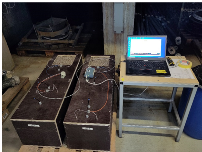
Figure 4. Two medium-scale boxes used to test the performance of the BER technology at larger distances between the anode and the cathode. The box on the right has a longer distance between the anode and cathode electrodes.
